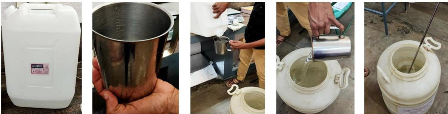
Step 3: Adding the required quantity of glycerine using a measuring jar into the solution and mixing it using a spatula
