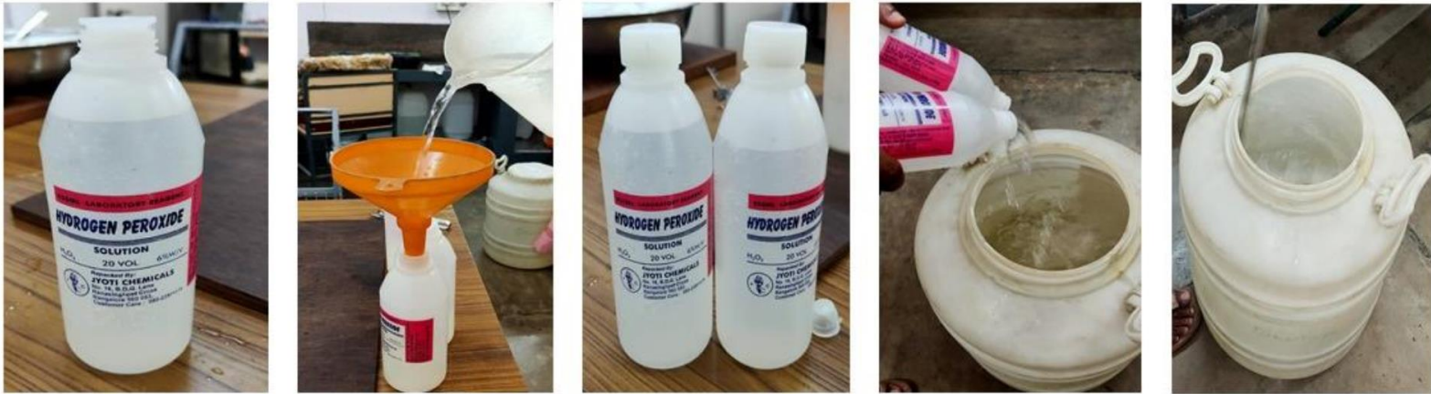
Step 2: Diluting 6% hydrogen peroxide to 3% using equal quantity of sterile distilled water and adding it to ethanol followed by mixing using a spatula
