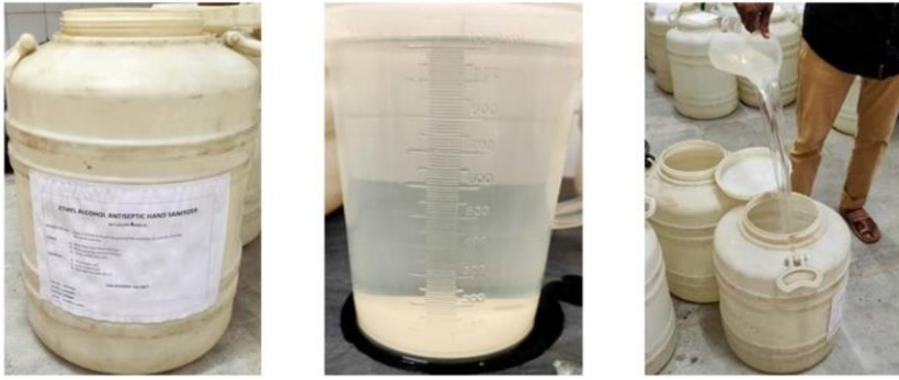
Step 1: Pouring required quantity of ethanol into a plastic drum using a measuring jar
